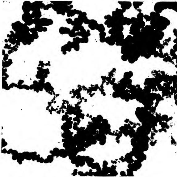
Figure 1. Semi-reinforcing furnace black before Cottrell agglomeration. (25,000x)
