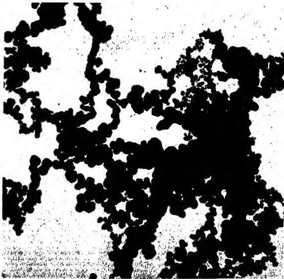
Figure 2. Semi-reinforcing furnace black after Cottrell agglomeration. (25,000x)
