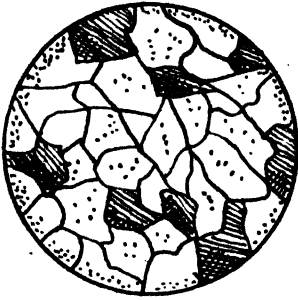
FIG. 15.—Sketch of the grain formation of mild steel.
