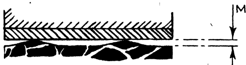
FIG. 60.—Sketch showing effect of macro surface on maximum bearing area ( M ).
