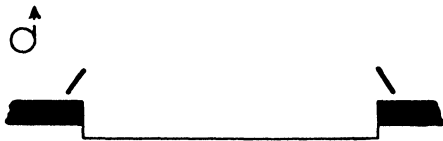
FIG. 163. PLAN: STAGE UNOBSTRUCTED WHEN CYCLORAMA CLOTH IS ROLLED UP
