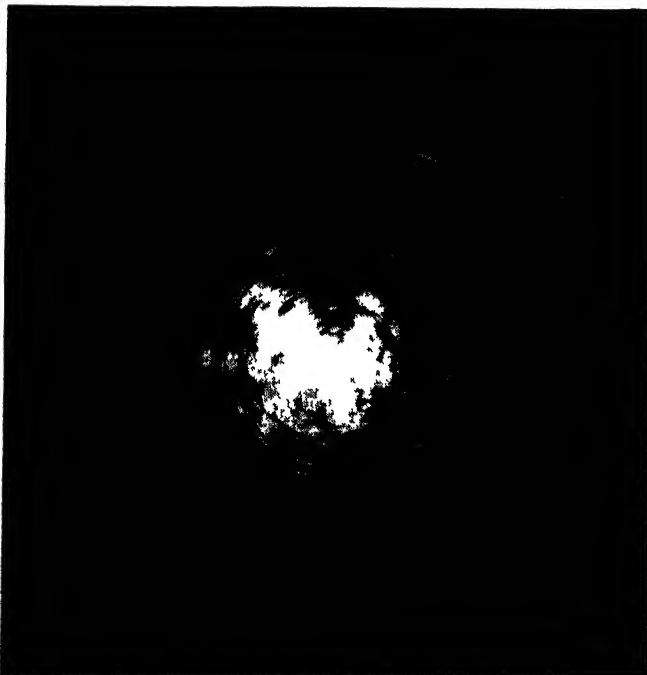
FIG. 14-7.—PPI photograph showing sector blanking due to radome wall reflections.
