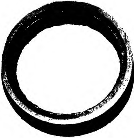
Figure 108. Uniform dezincification of brass.
