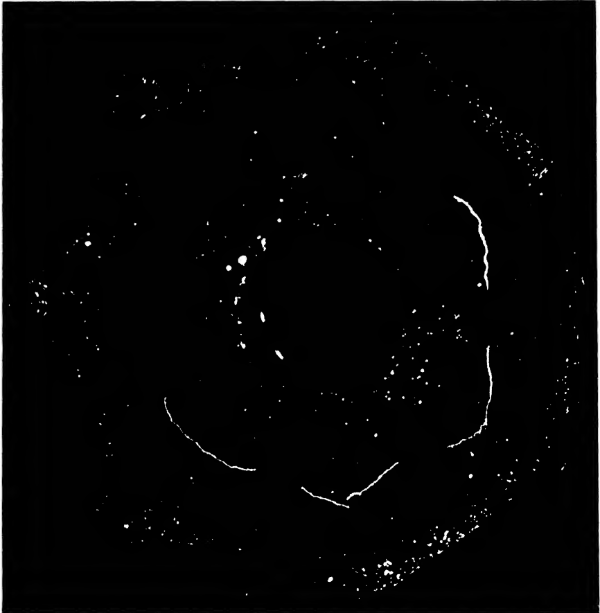
Figure 153. Zyglo indications of cracks and porosity.
