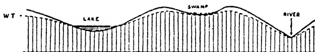
FIG. 23. — Diagram showing the relation between Topography and Water-table in a Homogeneous, Permeable Rock.
