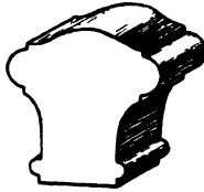
Fig. 101. Cross Section of Handrail Showing Top Shaped to Fit the Hand and the Bottom Flat to Receive the Balusters
