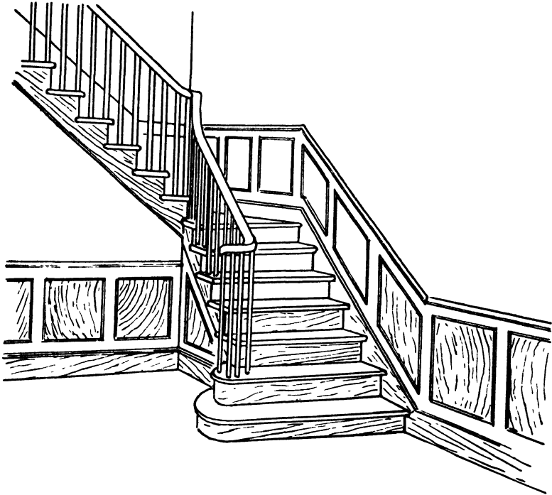
Fig. 106. Staircase with a Curved Handrail Forming Bottom Newel
