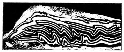
**B.** Experimental production of a series of parallel thrusts within closely folded strata (after Willis).
