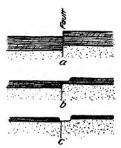
F10. 43. — Diagrams to show how an escarpment originally on the upthrown side of the fault may, through erosion, appear upon the downthrown side.
