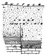
small faults in the rock basement may be masked at the surface through adjustments within the loose rock mantle.
