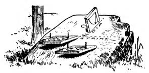
F10. 28. — Diagram to illustrate the manner of determining the strike of rock beds at an outcropping. a, a compass which has the cardinal directions in their natural positions; b, a compass with the east and west initials reversed upon the dial; c, home-made clinometer in position to determine the dip.
