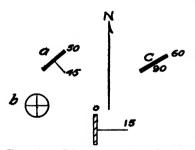
FIG. 29. — Diagram to show the use of T symbols to indicate the dip and strike of outcroppings. the dip angle by a figure at the end of the shank. It is the custom, also, to make the length of the shank inversely proportional to the steepness of the dip, so that in a broad way the attitudes of the strata may be taken in at a glance (Fig. 29). It is further of advantage to make the top of the T a double line, so that some symbol or color may show the correlations of the different expo-
