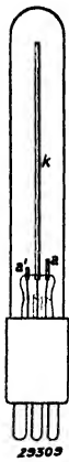
Fig. 320 Construction of the neon indicator tube 4662. k = cathode a = main anode a' = auxiliary or striking anode
