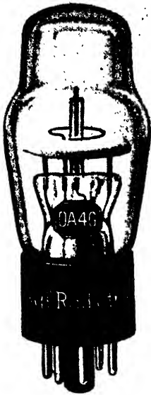
FIG. 4-30. Grid-controlled cold-cathode tube. (RCA.)
