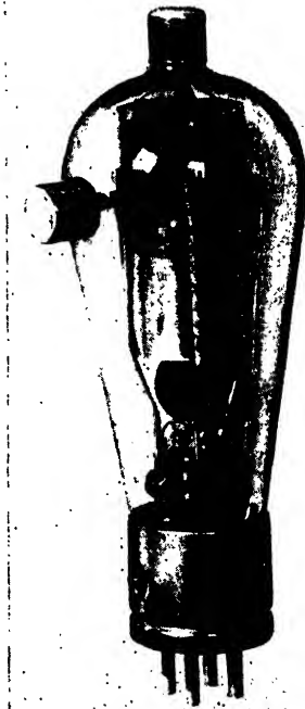
FIG. 4-32. A small, screen-grid thyratron. (General Electric Co.)
