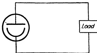
FIG. 5-16. Circuit using a photovoltaic cell to control a load which may consist of a relay, meter, or other device.
