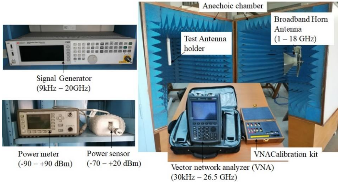
Fig.1.9 Antenna characterization facility at the parent institution
