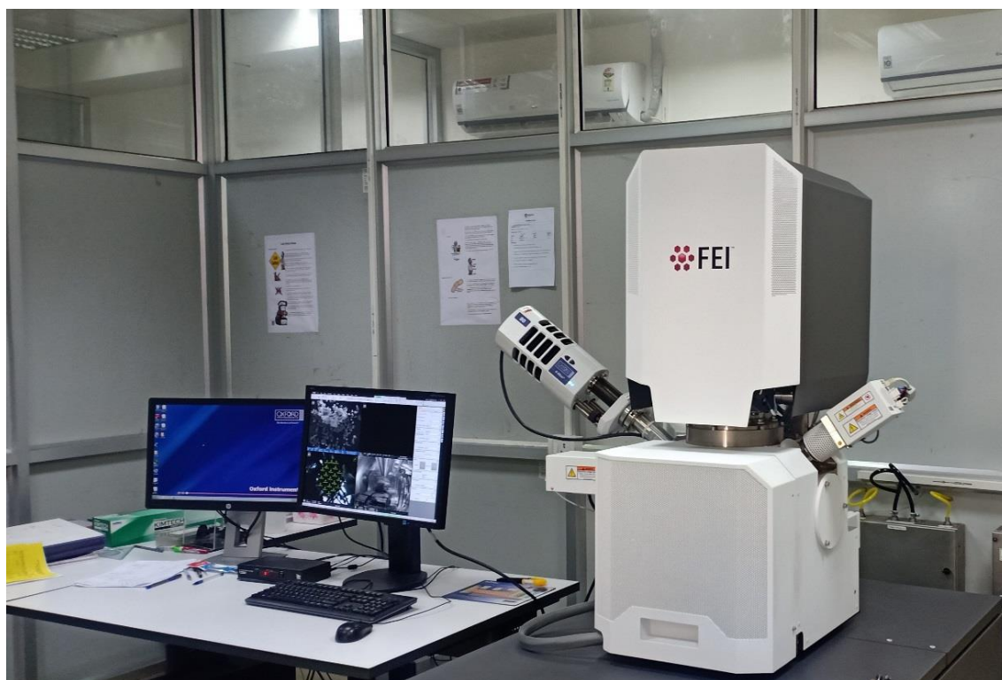
Figure 3.7: Field emission scanning electron microscopy (FESEM) attached with energy dispersive spectroscopy (EDS)
