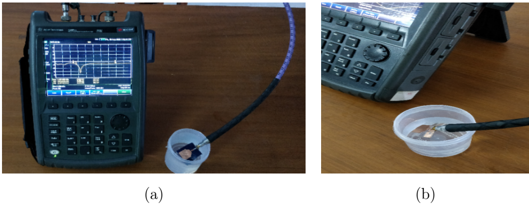
FIGURE 5.14: Measurement Set-up for wet condition, (a) Proposed antenna using Jean substrate, and (b) Proposed antenna using PDMS substrate
