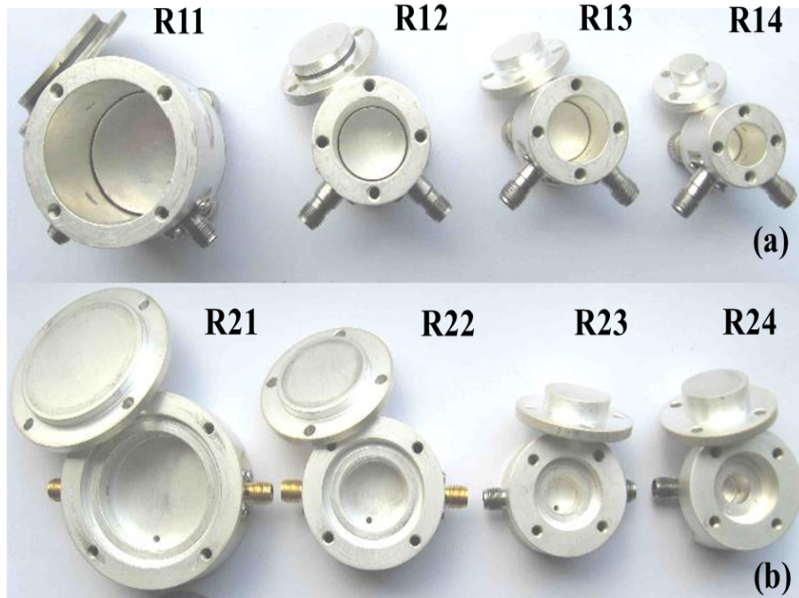
FIGURE 3.5: Family of optimized silver-plated measuring resonators: (a) TE -mode resonators R1 ( D_1 = 30, 18.1, 15, 10 mm) and (b) TM -mode resonators R2 ( D_2 = 30, 18.1, 10, 8 mm) which cover the frequency range of 6- 38 GHz (see Table 3.1).
