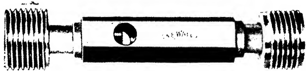
Fig. 99. -STANDARD AND EFFECTIVE "NOT GO" PLUGS (By courtesy of The Newall Engineering Co., Ltd.)
