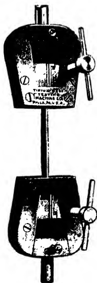
FIG. 65. WEDGE GRIPS FOR SHEET METAL TEST PIECES (Tinius Olsen Testing Machine Co.)
