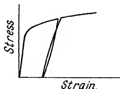
FIG. 216. HYSTERESIS LOOP OBTAINED WHEN LOADING AND UNLOADING BEYOND THE ELASTIC LIMIT
