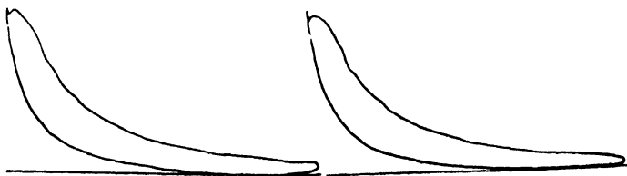
FIG. 16.—Coke-oven Tar with Petroleum Residuum for Ignition.
