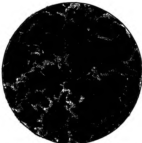
FIG. 23a.—Hypoeutectoid Steel ( \times 100 ) Containing About 0.40% C. Shows Ferrite (White) and Pearlite (Dark).
