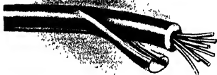
Low-voltage telephone wire, used by combat troops for distances up to 10 miles, combines desirable properties of polyethylene and nylon.
