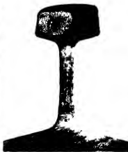
Transverse fissure in rail was discovered by the Sperry Detector before complete fracture of rail occurred.
