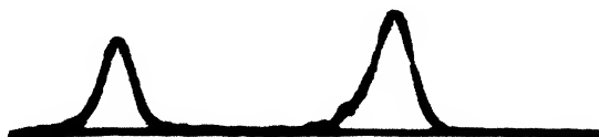
Fig. 6.—Gradient-curve photograph of the adsorption analysis of a mixture of 0.5% NaCl (right side) and 0.5% glucose (left side).
