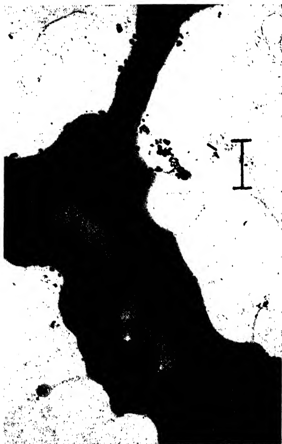
Fig. 11.—Electron micrograph of a thin film of rubber cement spread on water. Note carbon particles imbedded in film. (RCA Laboratories.)
