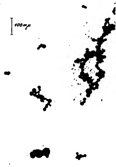
Fig. 15.—An electron micrograph of a mixture of two different sized gold particles. (By von Borries and Kausche (13).)
