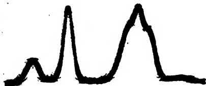
Fig. 11.—Adsorption analysis of a mixture of 0.5% rac. tartaric acid + 0.5% mesotartaric acid + 0.08 N sulfuric acid (left to right).
