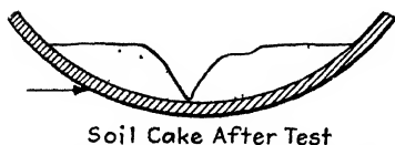
FIG. 36.—Diagram illustrating liquid-limit test.
