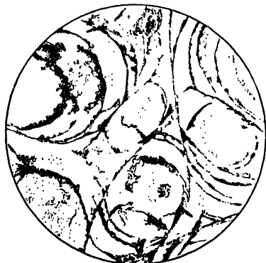
FIG. 39. Perlitic cracks in glass as seen in thin section under the microscope (see Chapter XXVII).
