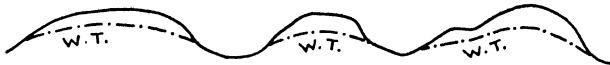
FIG. 74. Position of water table (dot and dash) in a hilly country made of permeable material.
