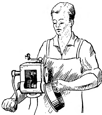
FIG. 9,817.—Wiring machine and its operation.
