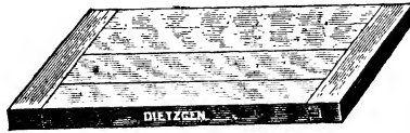
FIG. 1,481.—Dietzgen white pine drawing board with tongue and groove end ledges. This board has two drawing surfaces. Standard sizes: 12 × 7; 16 × 22; 20 × 24½; 20 × 26; 23 × 31; 31 × 43 ins. A good size for the beginner and for ordinary use is the 16 × 22 ins.
