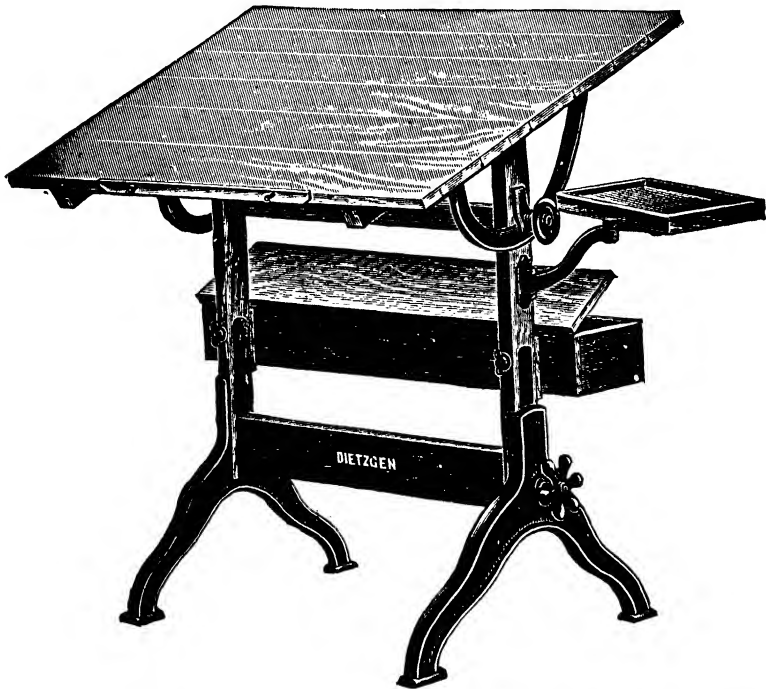
FIG. 1,482.—Dietzgen Eureka adjustable drawing table. Hardwood frame, iron legs, pine wood board having hardwood ledges. Height adjustment 32 to 40 ins. The wheel clamp at right locks table when tilted to any desired angle.
