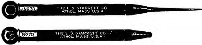
FIGS. 9,707 and 9,708.—Starrett pocket scribe, showing scriber in open and closed positions. The stock or handle is made from steel tubing knurled and nickel plated. The scriber blade is of steel, tempered, and is held by a knurled chuck. The scriber is reversible, telescoping into the stock and is held by a slight turn of the chuck so that the point is protected inside the stock when not in use as in fig. 9,708.
