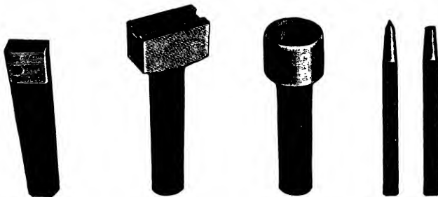
Figs. 9,855 to 9,859. —Tinner's hand tools 2. Fig. 9,855, rivet set and headers; fig. 9,856, grooving tool; fig. 9,857, hollow punch; figs. 9,858 and 9,859, solid punches.
