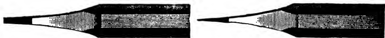
FIGS. 1,520 and 1,521.—End and side views of drawing pencil with lead sharpened "wedge shape."
