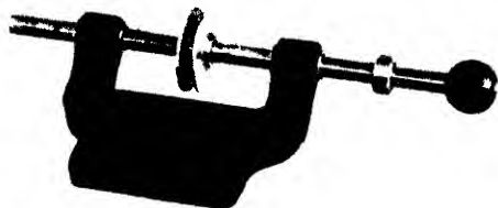
FIG. 91.—Simple precision or toolroom grinding spindle.
