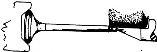
FIG. 20A.--Driving valve by friction cone against the head.
