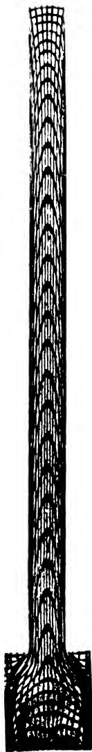
FIG. 97.- A billet of tin extruded at 140° C. from a cold container, bringing out the effect of a temperature gradient. (Cf. Fig. 88 a.)
