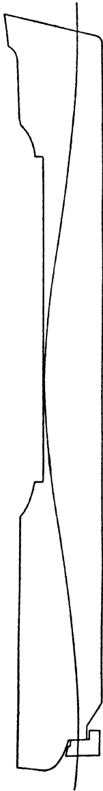
FIG. 248. Ship in Hogging Condition
