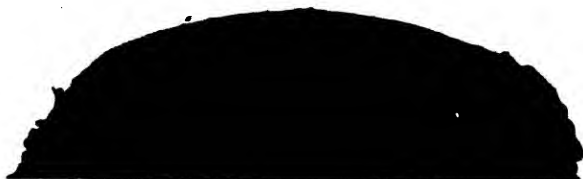
Fig. 4. Profile of Steel Pivot (No. 355) after 2,000,000 Revolutions in Contact with a Badly Orientated Sapphire Jewel (No. 37)
