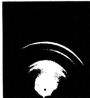
Fig. 4. Non-sharp Rings Indicating Unusually Short Random Crystalline Projections
