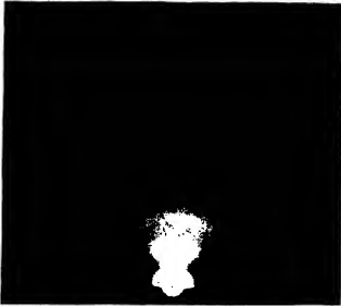
Fig. 5. Diffuse Halo Pattern, Typical of Liquid and Amorphous Surfaces
