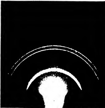
Fig. 3. Sharp - ringed Pattern Yielded by a Surface covered by many Chaotically Disposed, Very Thin, but Relatively Broad Crystalline Spikes
