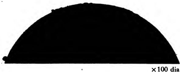
Fig. 3. Profile of Steel Pivot (No. 446) after 50,000,000 Revolutions in Contact with Diamond Jewel (No. 88)
