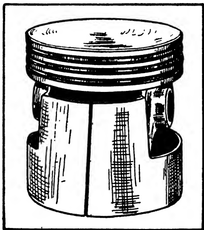
Fig. 42.—A Typical Aluminium Alloy Piston.
