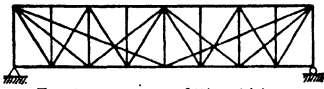
Tension members of Wrought Iron Compression members of Cast Iron. (A) Fink Truss (1852-76)
