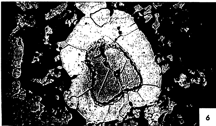
Micro. 15.6. Diffusion of Zn into Cu powder; \times 1,000 . Zn and Cu powders were heated together (without pressing) at a temperature at which no melting occurred and the loose powders did not sinter. The large particle shows a core of copper, a narrow zone of \alpha and a wide zone of \beta brass. Small particles in this photograph have been completely converted to the \beta phase. All these structures resulted from an inward diffusion of zinc, in the form of a vapor, from the surface of the copper particles.
