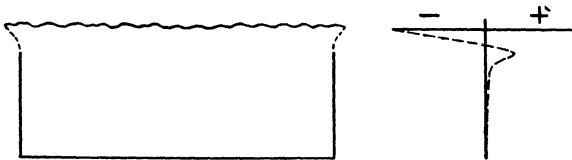
FIG. 6.11. Shot peening of the immediate top surface of the block (left side) tends to spread it. Rigidity of the metal underneath prevents bending or spreading; thus the surface is in compression (right-hand schematic stress plot) with a balancing layer underneath in tension.
