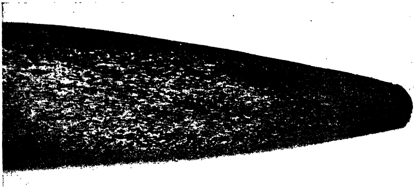
FIG. 6.8. Macrostructure of a longitudinal section of an aluminum alloy 25ST propeller as hot-forged and heat-treated, showing grains retained in elongated shapes by insoluble microconstituents and a finer grained structure nearer the surface, resulting from a lower hot-working temperature; \times 6 ; hot NaOH etch followed by \text{HNO}_3 dip.
