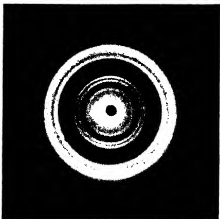
FIGURE 20-5 Typical powder photograph. Hexanolamine myristate, monochromatic radiation, from the Stanford laboratories of the author.
