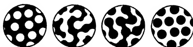
FIGURE 2-10 Diagram showing how an emulsion reverses. Taken from Sutheim, "Introduction to Emulsions," through the courtesy of The Chemical Publishing Co., Inc., Brooklyn, New York.
