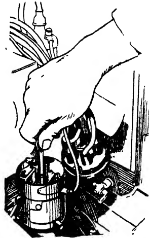
CHECKING DISTRIBUTOR POINT GAP
