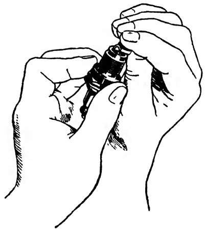
CHECKING SPARK PLUG GAP
