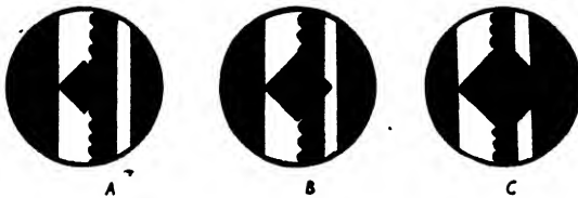
FIG. 138. ILLUSTRATING USE OF THIRD KNIFE EDGE FOR HARDNESS LIMIT VALUES
