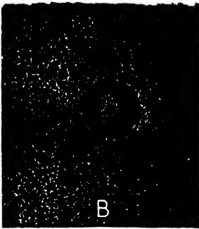
FIG. 159. MAGNIFIED PHOTOGRAPH OF IMPRESSION MADE BY NORMAL TIME TEST ON ANNEALED CARBON STEEL. (MAG. 50 TIMES)
