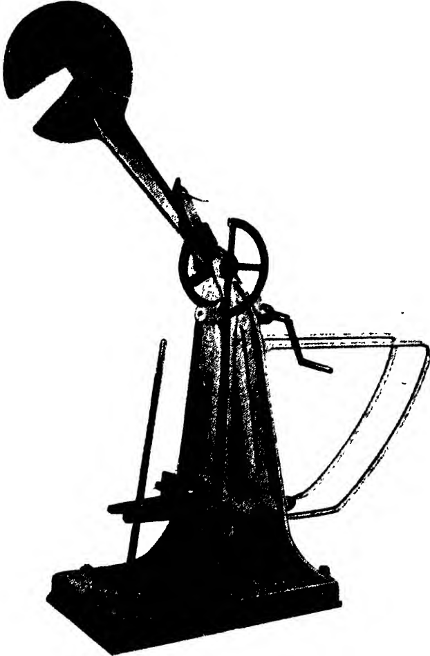
FIG. 237. THE CHARPY IMPACT MACHINE
