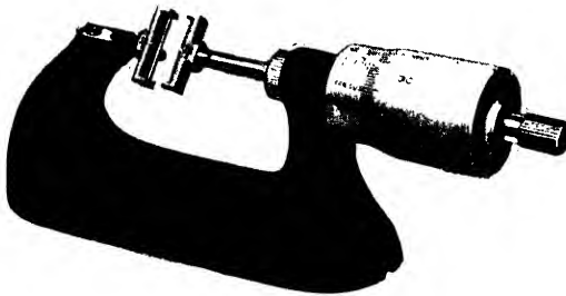
FIG. 91. THE TAVANNES THREAD-MEASURING MICROMETER (By courtesy of Adam Machine Tool Co., Ltd.)
