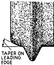
FIG. 11. SINGLE-RIB WHEEL WITH TAPER ON LEADING EDGE
