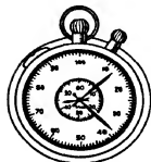
FIG. 116 STOP WATCH WITH TWO POINTERS (1) PER SINGLE OPERATION; (2) TOTAL TIME
