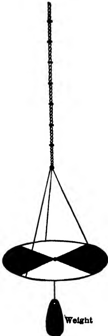
FIG. 52.—Disk for Comparing the Transparencies of the Water in Different Lakes.
