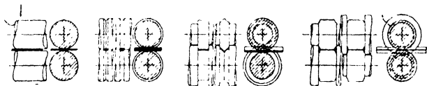
FIG. 18.—FORMS OF ROLLS USED IN THE ROLLING OF STEEL SECTIONS. Reproduced by permission and courtesy of Messrs. K. A. Skellon & Co., Ltd.
