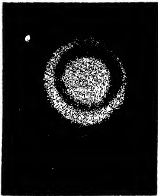
FIG. 2.—Diffraction of electrons on passing through a thin foil of matter.
