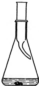
FIG. 1.—Apparatus for dissolving gallium in perchloric acid.
