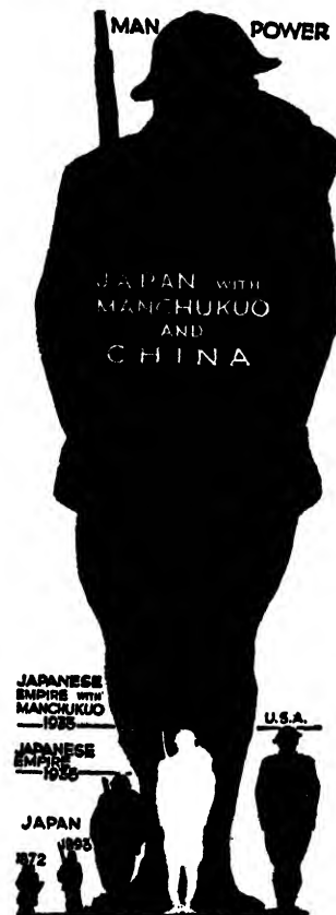
Fig. 206 Misleading use of pictorial graphs. The height of the silhouettes should be proportionate at least to the square root of the quantities.
