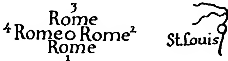
Fig. 126 City names are preferably centered below the symbol; second choice is to right or above. If it has to go on the left, it should be slightly above or below the symbol.
