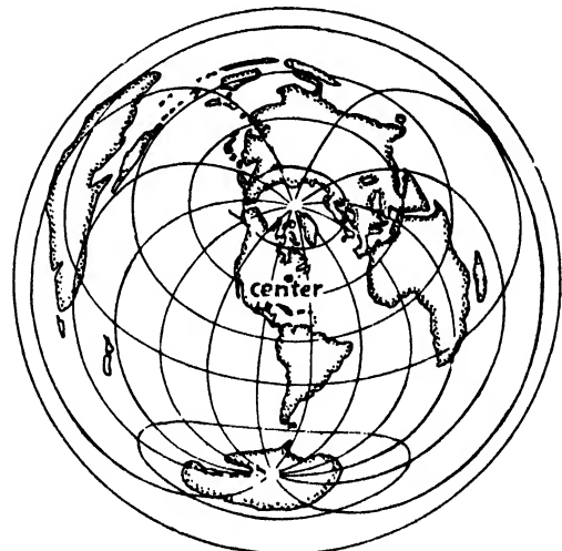
Fig. 71 In the azimuthal equidistant projection, every point is at its true distance and in the right direction from the center. (C. S. Hammond & Co.)
