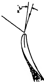
FIG. 4.20. Stalling due to separation at high positive incidence.
