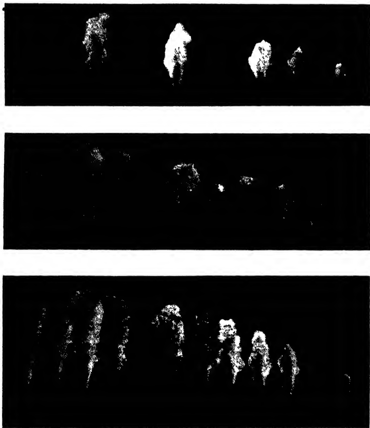
FIG. 11.—PHOTOGRAPHS OF SPRAY DEVELOPMENT.
