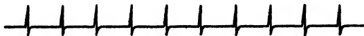
Fig. 5.45—For a time-calibrating scale, pulses of some such form as this are more convenient and precise than plain sine waves
