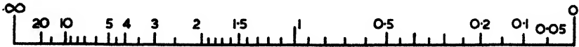
Fig. 5.7—Scale of the Fig. 5.6 type of ohmmeter, requiring only to be multiplied by R to indicate the resistance connected at “ x ”
