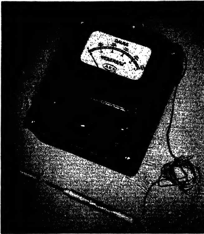
Fig. 10.14—A.E.I. direct-reading flux-meter, employing the Hall effect in germanium. The point of the probe is held in the magnetic field to be measured. (Associated Electrical Industries Ltd.)
