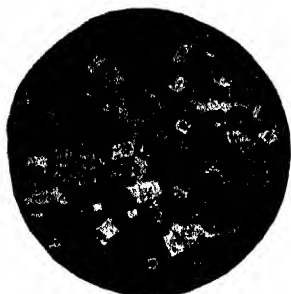
FIG. 130.—Microscopic section of chiascolite schist. The chiascolite crystals contain inside them some of the impurities of the rock, arranged more or less parallel to their outlines (about \frac{1}{2} ).
