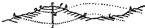
FIG. 1.—To show how the composition of rocks at a considerable depth may be ascertained from observations at the surface. a , b , g , h , i , k , seams of coal.
