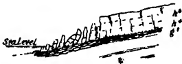
FIG. 39 a .—Section of the landslip of Axmouth, Devon. A^1 =Lias clay; A^4 =Greensand; B^4 =Chalk.
