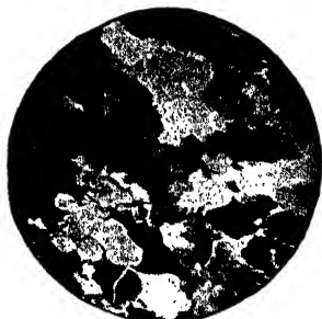
FIG. 132.—Microscopic section of granulite, to show the interlocking of the grains of quartz and felspar; taken with polarised light (about \frac{1}{2} ).
