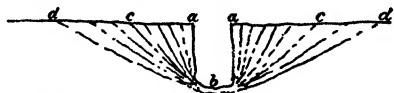
FIG. 29.—To show the successive stages in the opening out of a river gorge until a V-shaped valley is produced.
