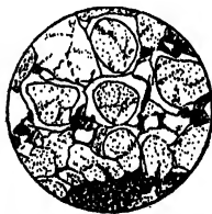
FIG. 135. — Microscopic section of quartzite from Little Caradoc, Shropshire. The original grains (slightly tinted) are to be seen inside the new growth of quartz at their edges (about \frac{1}{2} ).
