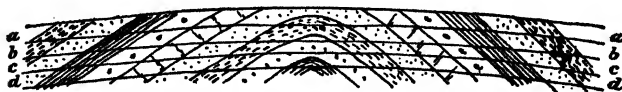
FIG. 289.—An anticline slowly rising and denuded by the sea as it rises, producing in succession the surfaces aa , bb , cc , dd .
