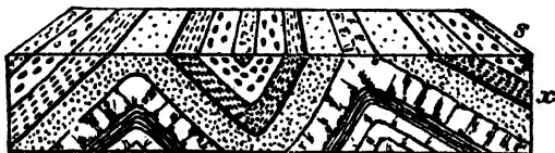
FIG. 68a.—Diagrammatic scheme of section ( x ) and outcrop ( s ) of the folds seen in the preceding figure.
