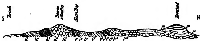
FIG. 256.—Section across the Isle of Wight, h^1 =Wealden strata; h^2 =Lower Greensand; h^3 =Gault; h^4 =Upper Greensand; h^5 =Chalk; i^2 =Woolwich and Reading Beds; i^3 =London Clay; i^4 =Bagshot Beds; i^5 =Bracklesham Beds; i^6 =Barton Clay; i^7 =Upper Bagshot Beds; i^8 =Lower Headon Beds; i^9 =Middle Headon Beds; i^{8'} =Upper Headon Beds; i^{8''} =Osborne Beds; i^9 =Bembridge Beds; i^{10} =Hamstead Beds.
