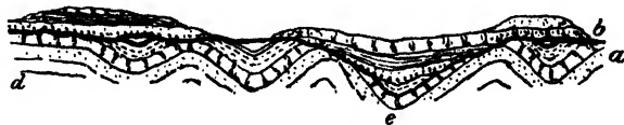
FIG. 153.—Unconformity of set of rocks a on set b ; deceptive at d and e , flagrant elsewhere.
