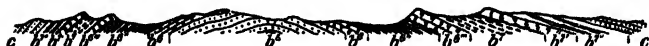
FIG. 180.—Section across the anticline of Woolhope, Herefordshire. b^b = Upper Llandovery Sandstone; b^b = Woolhope Limestone; b^{b''} = Wenlock Shale; b^{b'''} = Wenlock Limestone; b^7 = Lower Ludlow Beds; b^{7'} = Aymestry Limestone; b^{7''} = Upper Ludlow Beds; c = Old Red Sandstone.
