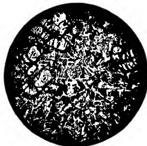
FIG. 9.—Microscopic section of ophitic dolerite. O=olivine; felspar, light needles; augite, half-tone; magnetite, black (magnified about 6 diameters, f).
