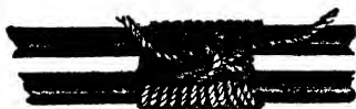
Fig. 12.—Lashing for Shear Legs. (For Tent Shears it is not Necessary to Take so many Turns)
