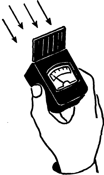
FIG. 2.—Light waves, indicated by arrows, cause photoelectric cell to react, registering intensity of light on calibrated scale.
