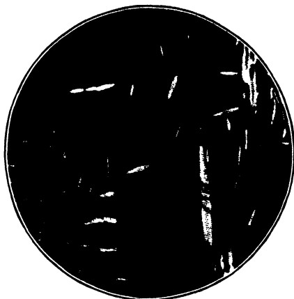
FIG. 62. Ramie fiber fragments after dissolving of acetylated portions. Hess and Schultze.
