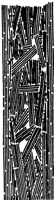
FIG. 40. Arrangement of macromolecules in artificial cellulose fibers. Staudinger and Jurisch.
