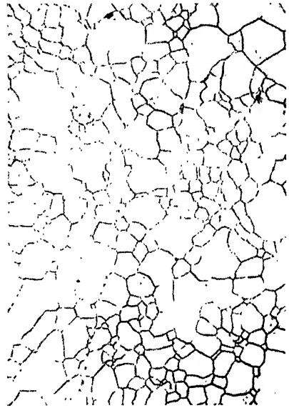
FIG. 131. — GRAIN SIZE OF A HARDENED EUTECTOID STEEL (MARTENSITIC STRUCTURE) REVEALED BY OXIDATION OF THE GRAIN BOUNDARIES AT THE SURFACE OF THE PIECE. (Etched with 15% HCl in ethyl alcohol.) X100. (Courtesy of Harry Tobin.)
