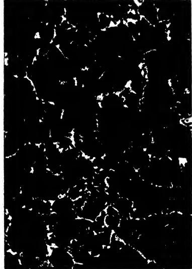
Left. FIG. 126. — 0.50% CARBON STEEL COOLED SLOWLY FROM 1560° F. (Etched with picral.) Rockwell "B" 92. X500.
