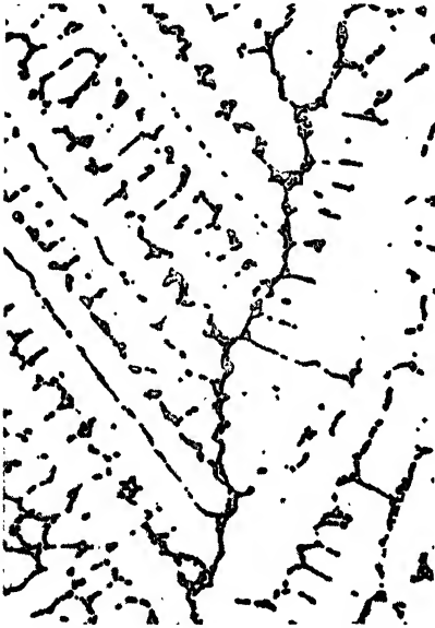
Left. FIG. 36.—HIGH PURITY ALUMINUM ALLOY CONTAINING 8% COPPER, AS CAST. (Etched with 0.5% HF in water.) X100. (Courtesy of the Aluminum Company of America.)
