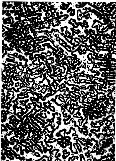
Left. FIG. 69. — PHOSPHOR BRONZE CONTAINING 92% CU-8% SN. AS CAST. (Etched.) Rockwell "B" 47. X100.
