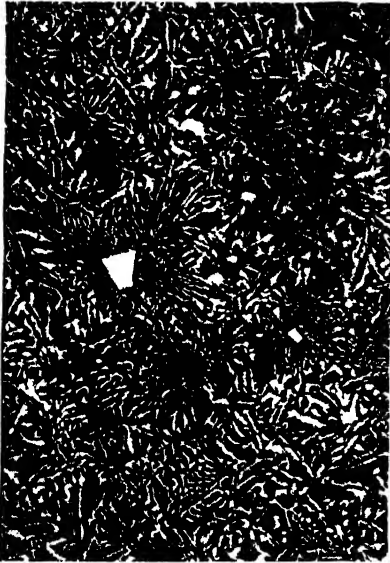
Left. FIG. 31. — LEAD BASE BEARING METAL CONTAINING 15% SB AND 3% SN. Brinell 18. X100.
