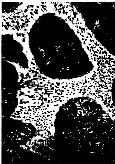
FIG. 211.—STADITE IN GRAY CAST IRON. (Etched with picral.) X1000.
