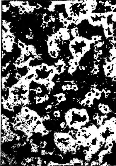
Left. FIG. 216. — PARTIALLY MALLEABLIZED WHITE IRON. (Etched with picral.) Brinell 183. X100.
