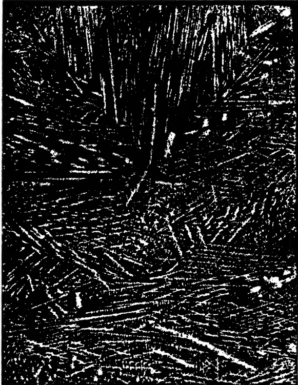
FIG. 165. — MACROSTRUCTURE OF A STEEL CASTING. (Etched in a boiling solution of 50% HCl-50% H 2 O, then repolished lightly.) X3. (Courtesy of H. S. Jerabek.)
