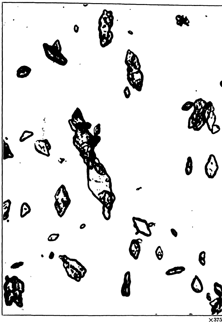
FIG. 18. Tobias Acid. Slow Agitation. (Courtesy of Imperial Paper and Color Corporation, Pigment Division.)
