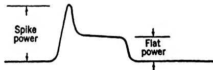
FIG. 2-30.—Envelope of the r-f pulse leakage from a TR switch as viewed with an r-f envelope viewer.
