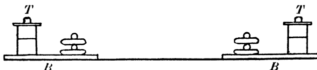
FIG. 143.—Clamp for fine wires.
